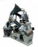
Creating and measuring forces to simulate and to test real time fatigue of the car suspensions taking into account a maximum of vehicle dynamics and creating different test lands
